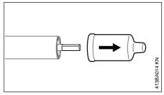
Pull the protective caps off the ends of the shaft and keep them in a safe place for later use – see "Storing the Machine".
